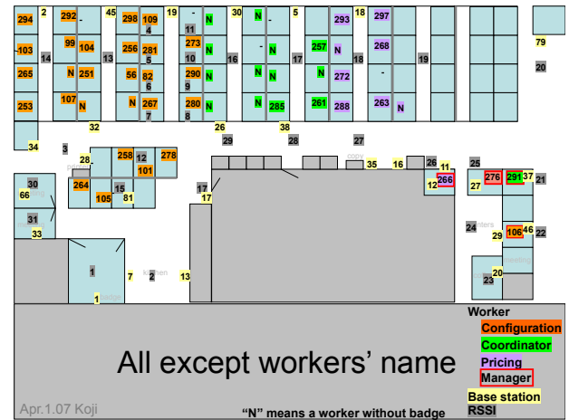
Figure 1: The configuration, coordination, and pricing branches in the organization each have their own spaces. Each participating employee was assigned a badge with a unique ID, and base stations with unique IDs were placed at fixed locations for time-sampling data records and for localization.
