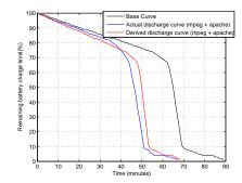
Fig. 8. Base curve together with discharge curves (actual and derived) for the new HP laptop (left) and old Dell laptop (right)
