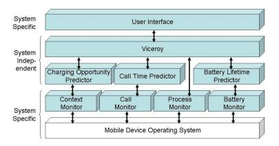
Fig. 2. CABMAN system architecture
